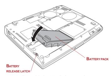
Figure 6-2 Securing the battery pack
